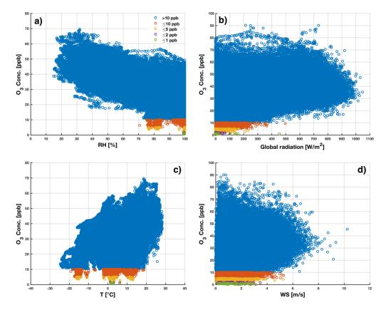
Figure 7. Ozone concentrations vs. a) relative humidity (RH), b) global radiation, c) temperature (T), and d) wind speed. Data were from the 16.8-m measurement level, with an exception of the global radiation data from 18 m.
