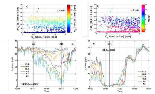
Figure 9. The ozone concentration difference between 67.2 and 4.2 m vs. the ozone concentration ( $\leq$  2 ppb) at 4.2 m, a) colour-coded by ozone concentrations at 67.2 m and b) colour-coded by month. c) A near-surface depletion event on September 14-15<sup>th</sup>, 2009. d) A full-profile depletion event on October 23<sup>rd</sup>, 2006. The vertical black lines indicate the sunrise (SR) and sunset (SS) times.
