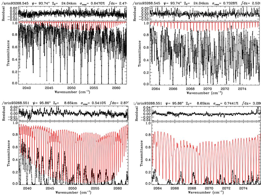
125 **Figure 1.** Examples of spectral fits to MkIV balloon spectra measured at 24.0 km (top) and 8.7 km (bottom) tangent altitude. The left-hand panels show fits to the P-branch. The right-hand panels show fits to the R-branch. Black points represent the measured spectra. The black line is the fitted calculation. The red line shows the OCS contribution to the fitted calculation.
