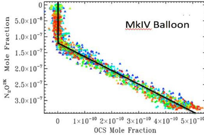
740 **Figure A.1.** The MKIV balloon OCS-N<sub>2</sub>O<sup>2K</sup> relationship color-coded by year and the fitted
