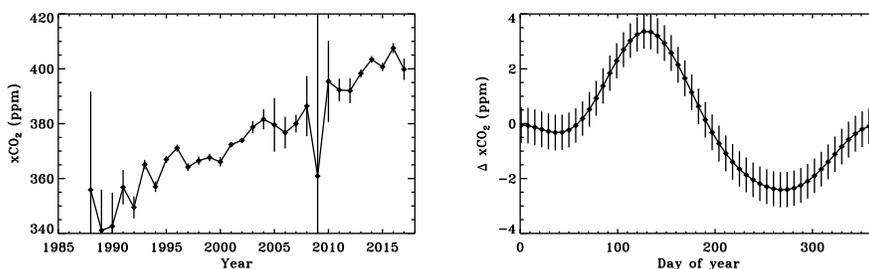
475 **Figure 7.** Decomposition of MKIV ground-based measurements of xCO<sub>2</sub> into a long-term secular trend (left) and a seasonal cycle (right). Years with little data, or with inconsistent xCO<sub>2</sub> values, have large uncertainties. The seasonal cycle has its peak around day 130 and its maximum rate of decrease around day 185.
