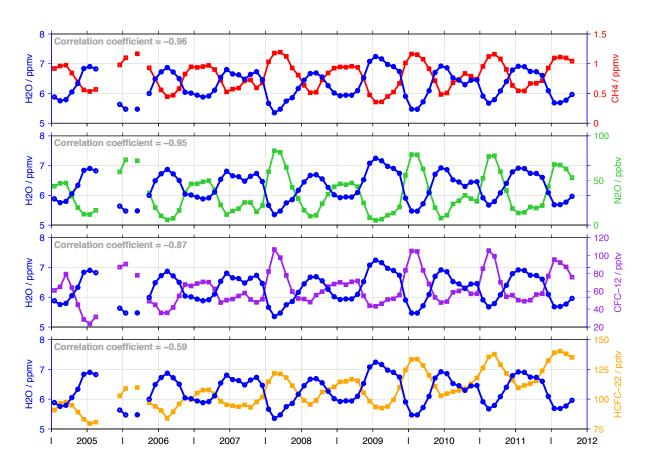
Figure 6. Comparison of the water vapour time series (blue, always left axis) with the time series of methane (red), nitrous oxide (green), CFC-12 (purple) and HCFC-22 (orange). All data consider MIPAS observations at 2.7 hPa for the latitude band from 18.5°S to 13.5°S. The correlation between the time series is indicated in the upper left corner.
