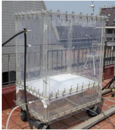
Figure 1. Photo (left) and schematic (right) of the quasi-atmospheric aerosol evolution study (QUALITY) chamber
