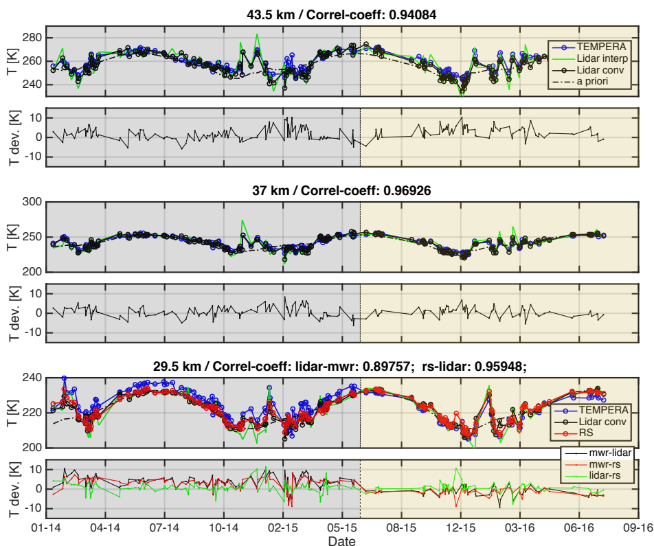
Figure 12. Stratospheric temperature evolution from TEMPERA, lidar and RS. Different background colors are used to distinguish between period 1 and 2 (gray and light brown, respectively).
