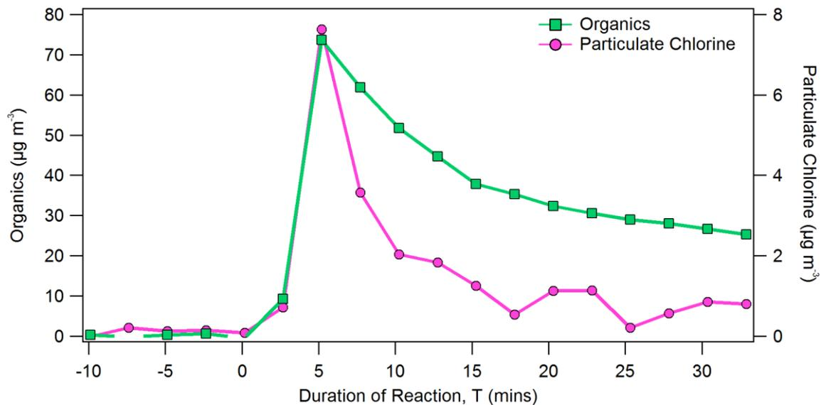
**Figure 4:** Measurements of particulate organics and chlorine from Exp. A8, not corrected for wall losses. UV was turned on at T = 0 mins. Apparent particulate chlorine concentration rapidly decreased to near-background levels while significant suspended OA mass remained. This rapid decrease is likely a measurement artifact due to build-up of chlorinated compounds on the vaporizer surface, see section 3.2 and S4.
