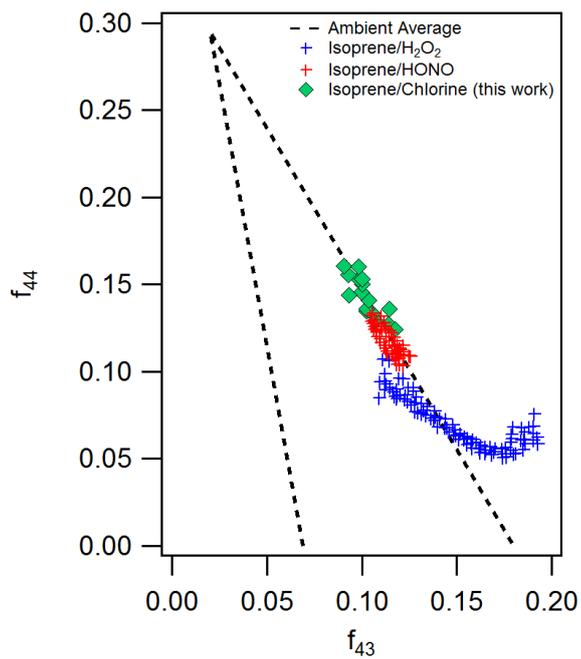
**Figure 3:** Extent of oxidation of SOA generated from chlorine-initiated reactions (Exp. C3, five-minute averages) compared to OH-oxidation of isoprene under low- and high- $NO_x$  (Chhabra et al., 2011). Area enclosed by the dashed lines represent typical ambient OA measurements (Ng et al., 2010).
