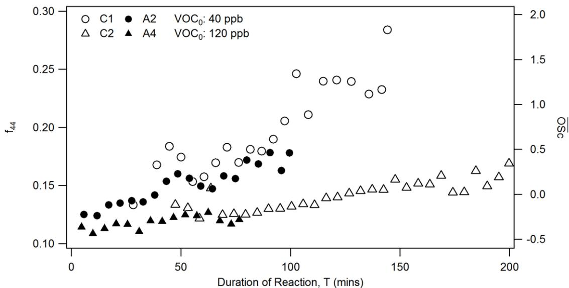
**Figure 2:** Comparison of SOA aging between two pairs (C1 and A2; C2 and A4) of initial and continuous chlorine injection experiments. The trend of  $f_{44}$  is consistent for each pair, regardless of chlorine injection method used. Higher initial isoprene concentration resulted in less oxidized organic aerosol (lower  $f_{44}$ ).  $\overline{OS}_C$  is estimated based on  $f_{44}$  (see section S2).
