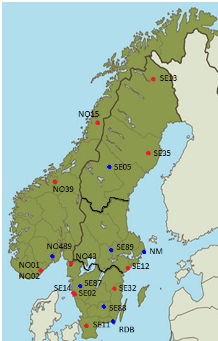
2 Figure 3. Instrumentation sites for hourly near-surface ozone concentration observations in 3 Sweden and Norway, which are used in the variational analysis. Red circles: sites with full 4 data coverage. Blue circles: sites with restricted data coverage. The subdivision of Sweden 5 into three regions (North, Central and South) follows county borders, as indicated by the fat 6 black lines.
