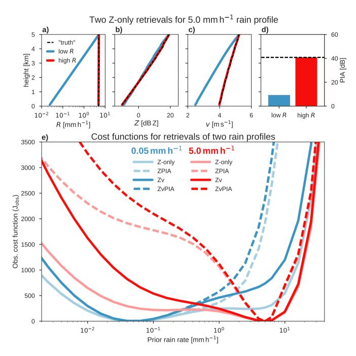
Figure 1. Above: Profiles of (a) retrieved rain rate, and (b) forward-modelled  $94\,\mathrm{GHz}$  radar reflectivity, (c) mean Doppler velocity and (d) PIA, for the two solutions to the retrieval from a synthetic profile; dashed lines show the values corresponding to the "true" profile of constant  $R = 5.0\,\mathrm{mm\,h^{-1}}$ .
