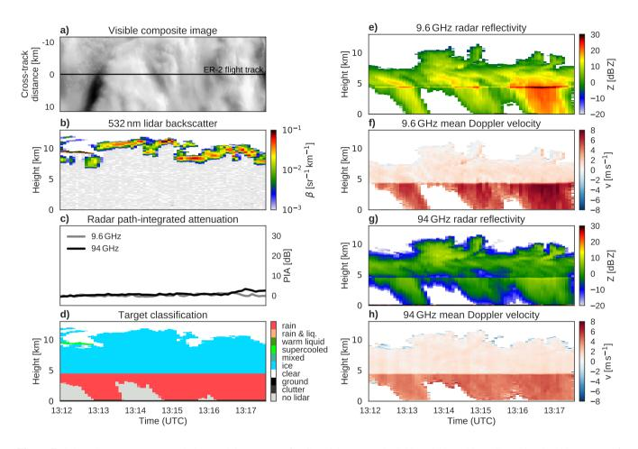
**Figure 7.** Selected measurements made by ER-2 instruments for Case 2 between 13:12:00 and 13:17:30 UTC on 22 July 2007 as part of TC4. The composite cloud image from MAS/MASTER visible channels (a), with the ER-2 flight track marked; 532 nm lidar backscatter (b); 9.6 and 94 GHz radar PIA (c); target classification from radar–lidar synergy (d); 9.6 GHz radar reflectivity (e) and mean Doppler velocity (f); and 94 GHz radar reflectivity (g) and mean Doppler velocity (h).
