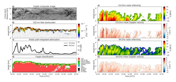
**Figure 10.** Selected measurements made by ER-2 instruments for Case 3 between 12:41 and 12:51 UTC on 29 July 2007 as part of TC4. Composite cloud scene (a) from MAS/MASTER visible channels, with the ER-2 flight track marked; 532 nm lidar backscatter (b); 9.6 and 94 GHz radar PIA (c); target classification from radar–lidar synergy (d); 9.6 GHz radar reflectivity (e) and mean Doppler velocity (f); and 94 GHz radar reflectivity (g) and mean Doppler velocity (h).
