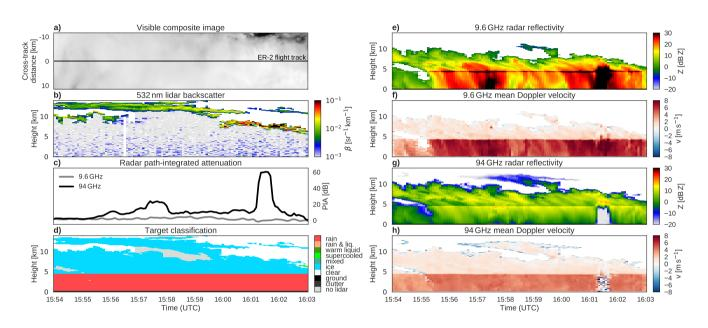
**Figure 3.** Selected measurements made by ER-2 instruments for Case 1 between 15:53 and 16:03 UTC on 22 July 2007 as part of TC4. Composite cloud scene (a) from MAS/MASTER visible channels, with the ER-2 flight track marked; 532 nm lidar backscatter (b); 9.6 and 94 GHz radar PIA (c); target classification from radar–lidar synergy (d); 9.6 GHz radar reflectivity (e) and mean Doppler velocity (f); and 94 GHz radar reflectivity (g) and mean Doppler velocity (h).
