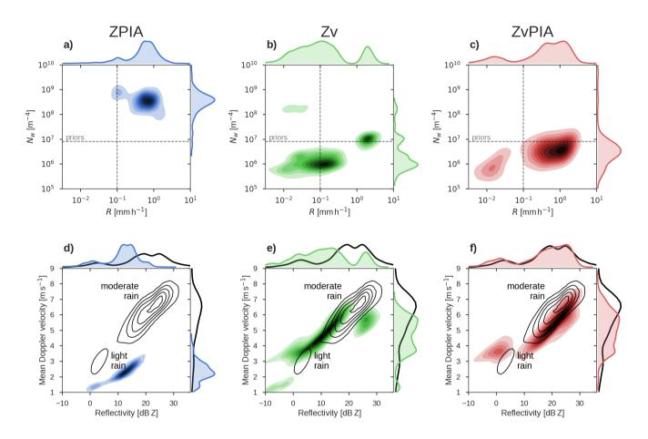
Figure 6. Joint (filled contours) and univariate (curves) kernel density estimation histograms of retrieved rain state variables R and  $N_w$  (a–c) and forward-modelled EDOP measurements (d–f) for ZPIA (a and d), Zv (b and e) and ZvPIA (c and f) rain retrievals during Case 1 on 22 July 2007. Dashed lines indicate the values of the prior state variables used in the retrieval. Black contours indicate the distribution of independent EDOP measurements; the major rain regimes are labelled.
