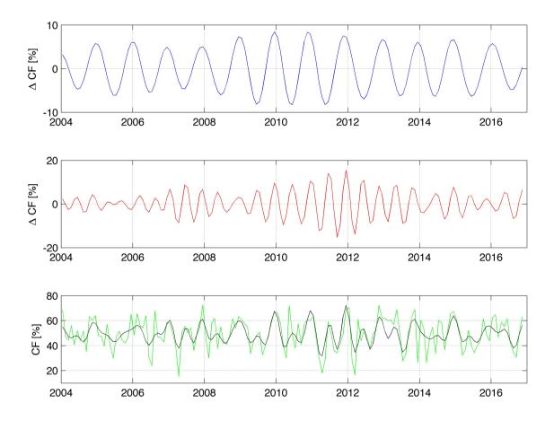
**Figure 3.** Annual oscillation (upper panel), semi-annual oscillation (middle panel) and time series of monthly means of CF (green line in the lower panel) derived from TROWARA measurements at Bern. The black line is the sum of the annual oscillation, the semi-annual oscillation and the total mean of CF.
