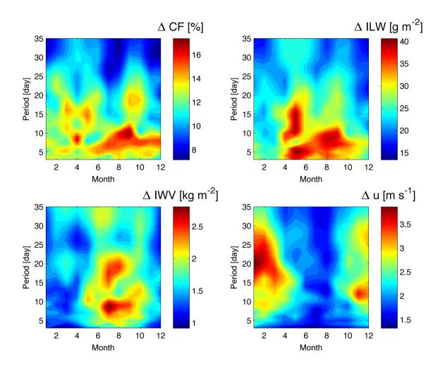
**Figure 8.** Climatologies of the short-term variability of CF, ILW, and IWV from TROWARA at Bern for the time interval from January 2004 to November 2016. In addition, we show the coincident climatology of zonal wind *u* from ECMWF operational reanalysis at 830 hPa (1.5 km altitude) above Bern. The amplitudes of the short-term variations in CF, ILW and IWV are enhanced from spring to fall. There are indications of a summertime 7 day-oscillation in CF, ILW and IWV.
