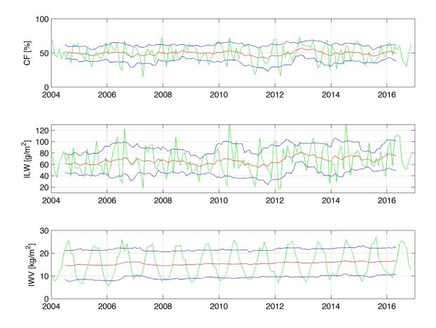
**Figure 1.** Time series of CF, ILW and IWV at Bern. The monthly means are given by the green lines while the red lines denote the annual means (12 months-sliding average with a step of 1 month). The blue lines shows the standard deviations of the annual means. Please note that a seasonal oscillation is only clear for IWV.
