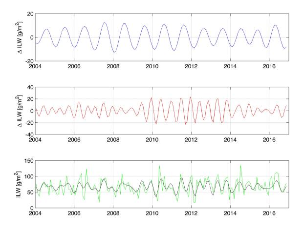
**Figure 4.** Annual oscillation (upper panel), semi-annual oscillation (middle panel) and time series of monthly means of ILW (green line in the lower panel) derived from TROWARA measurements at Bern. The black line is the sum of the annual oscillation, the semi-annual oscillation and the total mean of ILW.
