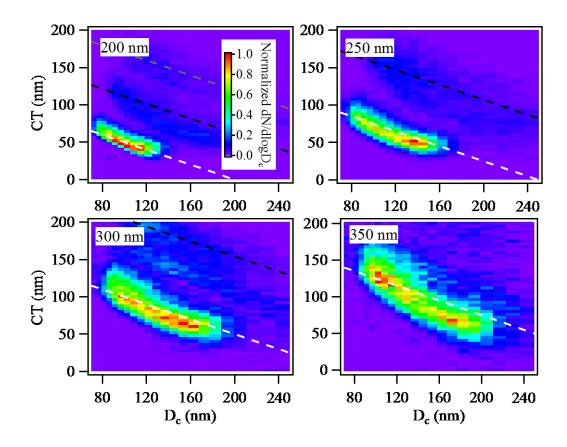
Fig. R13 (Figure S8 in the revised manuscript). Coating thickness (*CT*) of internally-mixed BC particles at 200-350 nm (selected by DMA1) as a function of rBC core size (*D*c). The dash line is  $CT=(D_{\text{selected}}-D_c)/2$ , i.e., the theoretic *CT*; the white, black and grey colors reflect the singly, doubly and triply charged particles.
