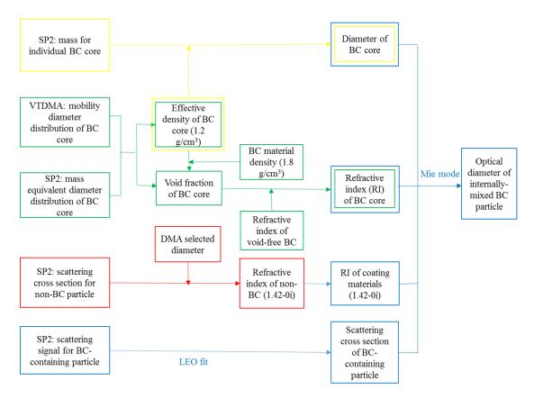
Fig. R2 (Figure. S2 in the revised manuscript). Schematic of optical size calculation for internally-mixed BC particle.
