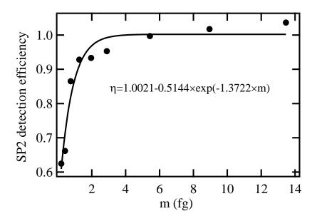
Fig. R8 (Figure S4 in the revised manuscript). The SP2 detection efficiencies ( $\eta$ ) in each BC mass-bin.
