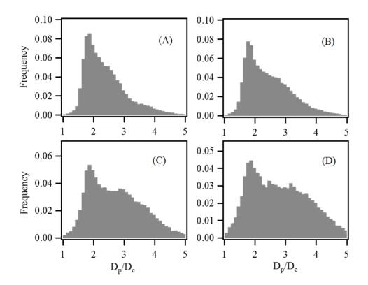
Figure. R10 (Figure. S5 in the revised manuscript). The frequency distribution of  $D_p/D_c$  ratio for internally-mixed BC with different mobility diameters ((A) 200, (B) 250, (C) 300 and (D) 350 nm) selected by DMA1.
