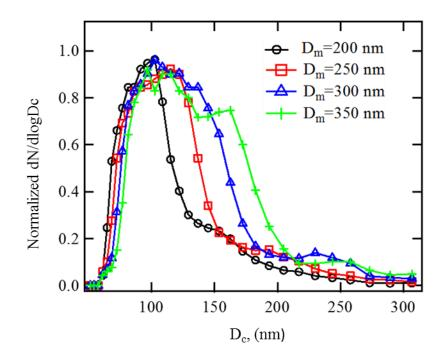
Fig. R12. (Figure S7 in the revised manuscript). The number size distribution of BC cores for internally-mixed BC.
