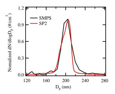
Fig. R1. The size distribution of PBL at 203 nm using SMPS and SP2 measurements.
