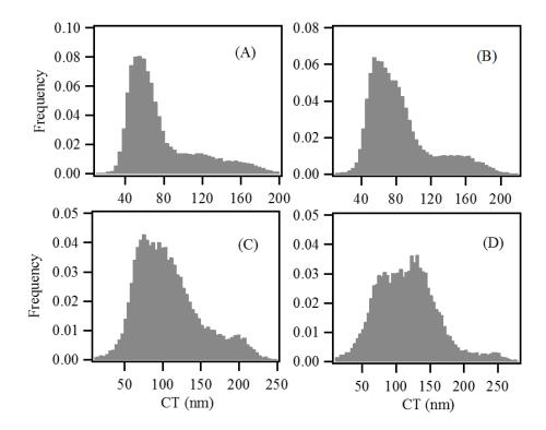
Figure. R9. (Figure 10 in the revised manuscript) The frequency distribution of coating thickness (CT) for internally-mixed BC with different mobility diameters ((A) 200, (B) 250, (C) 300 and (D) 350 nm) selected by DMA1.
