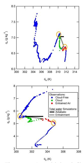
Figure 10. Conservative variables, water vapor content  $(q_v)$ , conservative in subsaturated conditions and derived from RH measurements) and equivalent potential temperature  $(\theta_e)$  identify mixing between cloud air and entrained air. Measurements are defined as cloud-free (blue), in-cloud (green) or entrained air sources (red). The orange circles highlight what is suggested to be the non-mixed sources of air.
