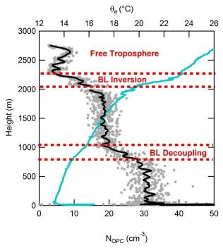
Figure 9. Flight 10 UAV vertical profile of OPC aerosol number concentrations (Dp > 0.5 um) (grey) with a 20 second running mean (black) and equivalent potential temperature ( $\theta_e$ , light blue) illustrate decoupling of the boundary layer. Incloud OPC measurements (2000 m- 2050 m) have been removed.
