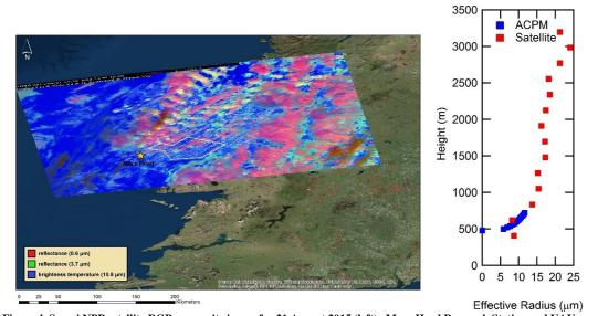
Figure 4. Suomi NPP satellite RGB composite image for 21 August 2015 (left). Mace Head Research Station and UAV flight location are indicated by the yellow star. The white polygon represents the zone for retrieving cloud properties – which is represented by the profile of cloud effective radius (right). Effective radius profiles are presented for both the Suomi NPP satellite (red) and the ACPM (blue).
