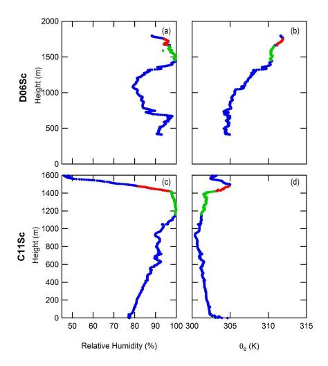
Figure 11. UAV vertical profiles of relative humidity (a, c) and  $\theta_c$  (b, d) for flights D06Sc and C11Sc, used in Figure 9. Profiles are defined as cloud-free (blue), in-cloud (green) or entrained air sources (red).
