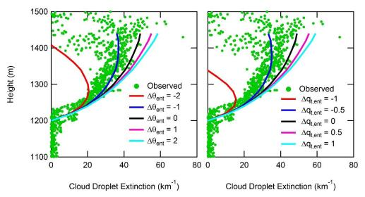
Figure 12. Sensitivity of simulated cloud extinction based on variability of entrained air potential temperature ( $\Delta\theta_{ent}$ ) and entrained air total water mixing ratio ( $\Delta q_{t,ent}$ ) for the C11Sc case. Black lines are equivalent to the adiabatic simulation with entrainment from Figure 7c.
