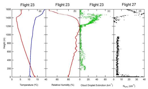
Figure 7. Vertical profiles of temperature, virtual potential temperature  $(\theta_v)$ , relative humidity, cloud droplet extinction and OPC total aerosol concentration. The figure consists of measurements collected from flights 23 and 27 on 11 August 2015 between 12:00 - 12:47 and 16:58 -17:33 respectively. The cloud level is between 12:00 m to 1480 m in flight 23, and lowered to approximately 980 m to 1280 m in flight 27. OPC measurements that occurred in the cloud have been removed.
