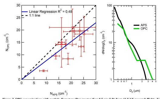
Figure~2.~OPC~concentrations~with~particle~diameters~(Dp)~greater~than~0.5~um~(left)~from~11~UAV~research~flights, listed~concentrations~viii.670 in Table 1, plotted against APS concentrations (Dp > 0.5 um) at Mace Head Research Station (red circles). Error bars represent ±1 standard deviation. The points are fit with a linear regression (blue line). OPC data was averaged between 40 and 80 m asl. Averaged OPC and APS number size distributions averaged for the 11 flights (right).
