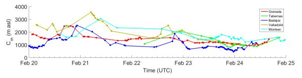
Figure 9. Time series of the integral of the particle backscatter coefficient for all stations (top panel) and time series of the center of mass of the backscatter profiles for all stations (bottom panel).
