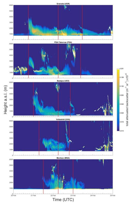
Figure 7. Ceilometer time series of total attenuated backscatter representing the evolution of the dust outbreak between 20 and 24 of February 2016 (the color scale is logarithmic). Red vertical lines indicate the time of the profiles in Fig. 8: First line of each site indicates the times for Fig. 8a, second line for Fig. 8b, and third line for Fig. 8c.
