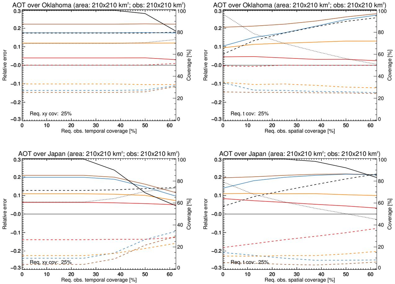
**Figure 14.** Monthly mean (dashed) and RMS (solid) of representation errors for an imager on a polar-orbiting satellite as a function of required spatial or temporal coverage of the observations. Results are shown for no collocation (brown), no collocation but using super-observations (dark blue), collocation to the day (orange), and finally model data collocated to the hour (red). Results for a repeat cycle of 1 day. Further explanation in Sect. 3.2.
