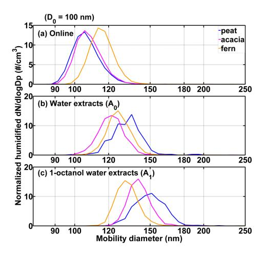
**Fig.2** Normalized number size distributions measured by the HTDMA ( $D_0 = 100$  nm; RH = 90%) of peat, fern and acacia burning particles. (a) online data, (b)  $A_0$ , and (c)  $A_1$ . For online data, peat burning particles are nearly non-hygroscopic, while fern burning particles are more hygroscopic. Aqueous extracts of peat burning particles are the most hygroscopic among the three types of biomasses. The x-axis is on a logarithmic scale.
