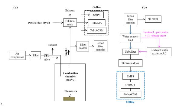
2 Fig. 1 Schematic diagrams of the laboratory experimental setups.
