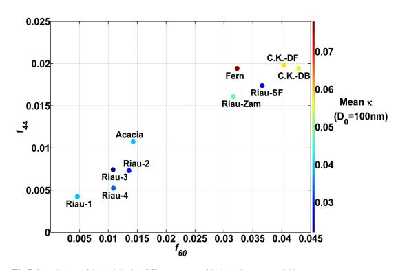
**Fig.7** Correlation of  $f_{44}$  and  $f_{60}$  for different types of Indonesian peat and biomasses.
