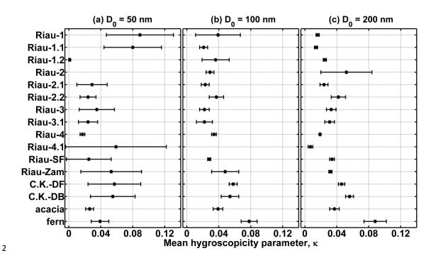
**Fig.3** Mean  $\kappa$  values of fresh Indonesian biomass burning particles measured for (a)  $D_0 = 50$  nm,
