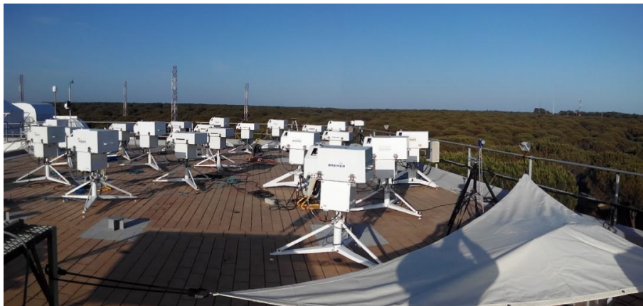
Figure 2. Panoramic view of the 21 Brewer spectrophotometers on the terrace of the El Arenosillo sounding station, Huelva, coming from Canada (1), Netherlands (2), United Kingdom (3), Switzerland (1), Finland (1), Greece (1), Denmark (2), Russia (1), Algeria (1) and Spain(7).
