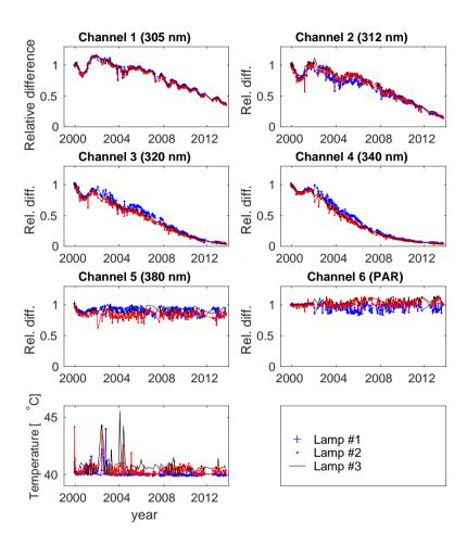
Figure 2. Lamp measurements at Marambio 2000-2013. The raw data of the lamp is divided by the mean of the three first measurements same as Fig. The temperature of the NILU-UV during the measurement is also shown 1 but for Marambio.
