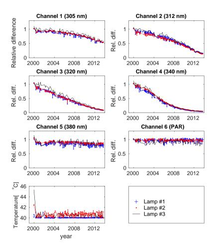
**Figure 1.** Lamp measurements at Ushuaia during 2000-2013. The raw data of the lamp is are divided by the mean of the three first measurements measurements. The temperature of the NILU-UV during the measurement is also shown.
