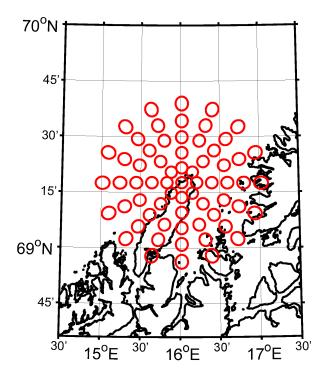
**Figure 1.** Projection of MAARSY beam positions for the multi-beam experiments during summer 2013. The red circles show the illuminated radar beam area assuming a beam width of  $3.6^{\circ}$  at 84 km altitude. The black lines are the shore line around the north Norwegian island Andøya.
