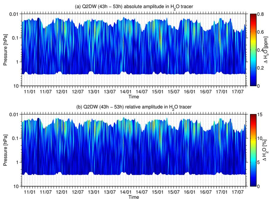
**Figure 2.** Evolution of absolute (a) and relative (b) Q2DW amplitude in water vapor data from the middle atmospheric water vapor radiometer MIAWARA in the time period from 1 October 2010 to 30 September 2017. The data product is shown in the altitude region where it can be regarded as reliable according to Fig. 1.
