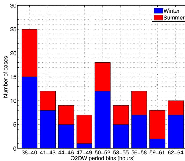
**Figure 6.** Histogram of Q2DW periods observed with the MIAWARA water vapor radiometer. Shown are the number of cases versus period bins with 3 h width in which Q2DW events could be identified. The selected criterion of a Q2DW event was a localized maximum in a monthly averaged H<sub>2</sub>O wave spectrum exceeding 0.15 ppm. The bar plots are stacked which divides them into winter (blue) and summer (red) groups.
