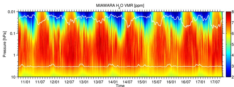
**Figure 1.** Water vapor volume mixing ratio [ppm] time series as measured by the MIAWARA microwave radiometer between October 2010 and September 2017. The horizontal white lines indicate at which pressure levels the measurement response drops below 50%. Clearly seen is the annual cycle in the mesosphere with a H<sub>2</sub>O maximum in summer. The measurement response is affected by tropospheric opacity which is higher in summer what leads to the observed variation in time.
