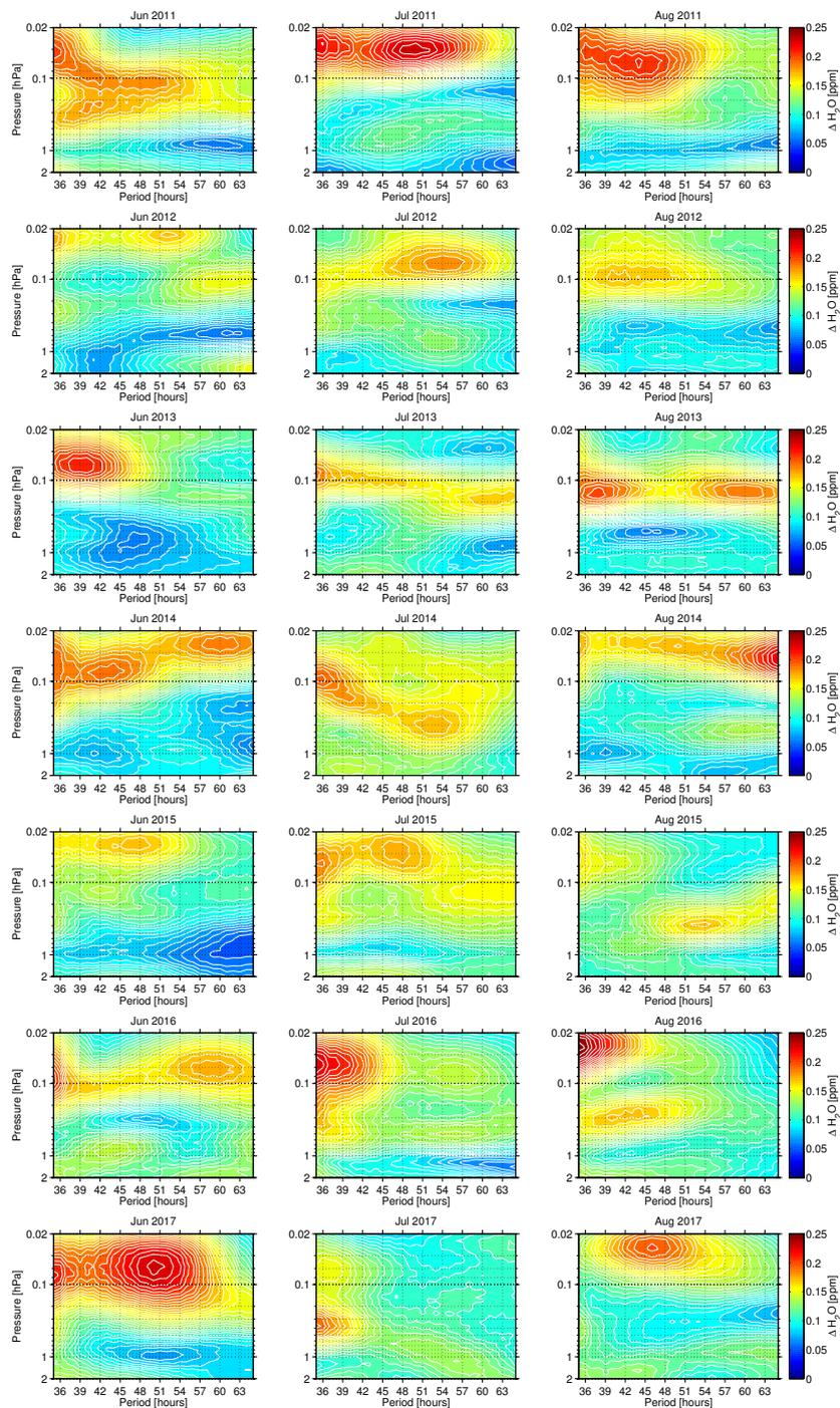
**Figure 3.** Monthly averaged water vapor wave amplitude spectra with periods between 35 and 65 hours in units of [ppm]. Presented are the months June (first column), July (second column) and August (third column) for the years from 2011 to 2017.
