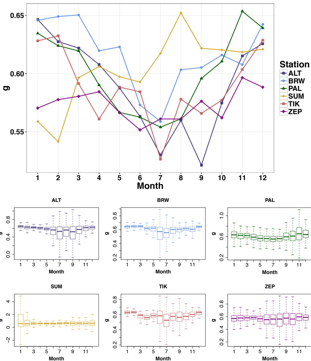
Figure 7. Seasonality of aerosol asymmetry parameter ( $g$ ) at all sites. Large plot shows monthly medians of hourly average  $g$  at 550nm at each station, subplots below show boxplots of  $g$  at individual sites with horizontal line at the median, edges of the box at 25<sup>th</sup> and 75<sup>th</sup> percentiles, and whiskers at 5<sup>th</sup> and 95<sup>th</sup> percentiles. Note that y-axes are difference on each plot.
