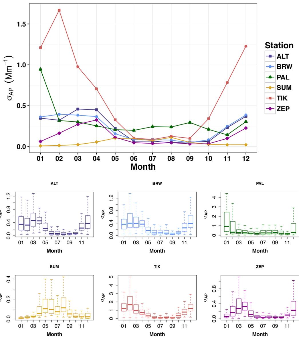
Figure 4. Seasonality of aerosol light absorption coefficient ( $\sigma_{ap}$ ) at 550nm at all sites. Large plot shows monthly medians of absorption in  $Mm^{-1}$  at each station, subplots below show boxplots of hourly average absorption at individual sites with horizontal line at the median, edges of the box at 25<sup>th</sup> and 75<sup>th</sup> percentiles, and whiskers at 5<sup>th</sup> and 95<sup>th</sup> percentiles. Note that y-axes are different on each plot.
