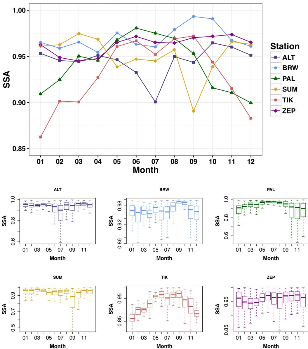
Figure 5. Seasonality of single scattering albedo (SSA) at all sites. Large plot shows monthly medians of hourly average SSA at 550nm at each station, subplots below show boxplots of SSA at individual sites with horizontal line at the median, edges of the box at 25<sup>th</sup> and 75<sup>th</sup> percentiles, and whiskers at 5<sup>th</sup> and 95<sup>th</sup> percentiles. Note that y-axes are different on each plot.
