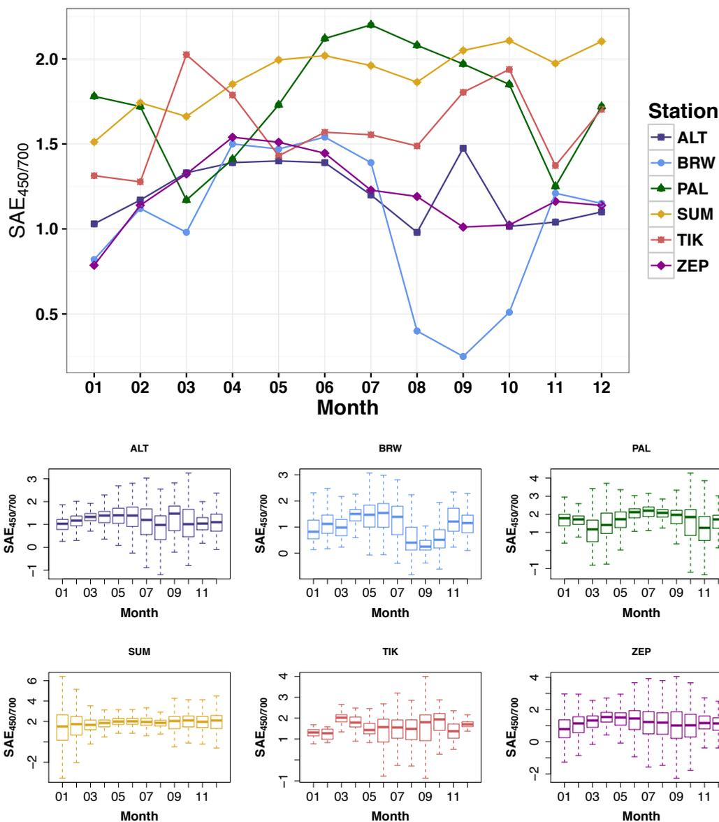
Figure 6. Seasonality of scattering Ångström exponent (SAE) at all sites. Large plot shows monthly medians of hourly average SAE at the 450nm/700nm wavelength pair at each station, subplots below show boxplots of SAE at individual sites with horizontal line at the median, edges of the box at 25<sup>th</sup> and 75<sup>th</sup> percentiles, and whiskers at 5<sup>th</sup> and 95<sup>th</sup> percentiles. Note that y-axes are different on each plot.
