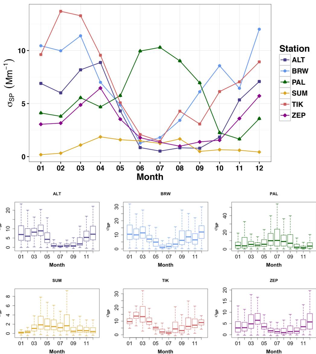
Figure 3. Seasonality of aerosol light scattering coefficient ( $\sigma_{sp}$ ) at 550nm at all sites. Large plot shows monthly medians of scattering in  $Mm^{-1}$  at each station, subplots below show boxplots of hourly average scattering at individual sites with horizontal line at the median, edges of the box at 25<sup>th</sup> and 75<sup>th</sup> percentiles, and whiskers at 5<sup>th</sup> and 95<sup>th</sup> percentiles. Note that y-axes are different on each plot.
