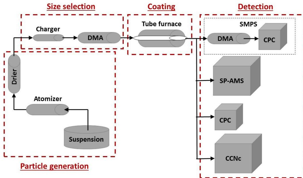
5 Fig. 1: Schematic of the experimental set up, including particle generation using an atomizer and a drier, size selection with a Differential Mobility Analyzer (DMA), coating and three types of measurements: CCN activity measurements using a Condensation Particle Counter (CPC) and a Cloud Condensation Nuclei Counter (CCNc), size distribution measurements by a Scanning Mobility Particle Sizer (SMPS) and particle composition analysis by a Soot Particle Aerosol Mass Spectrometer (SP-AMS).
