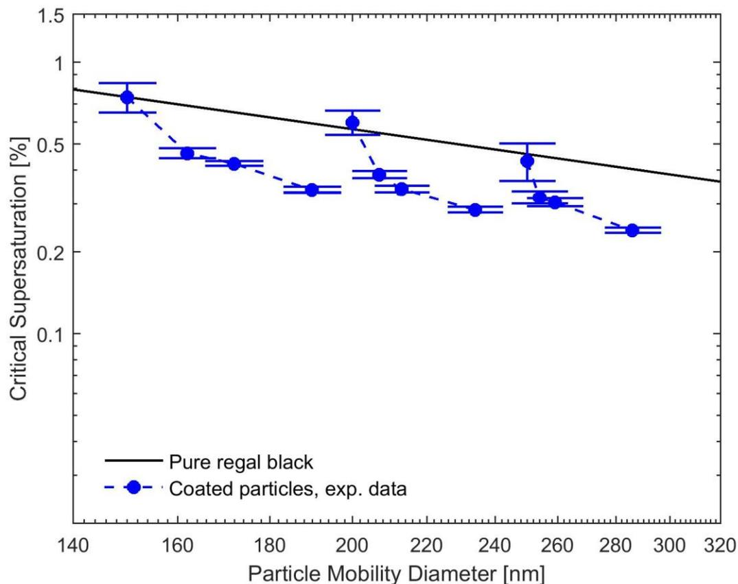
**Fig. 7: Experimental and theoretical critical supersaturations for coated BC by oleic acid for different particle mobility diameters. Black line represents the calculated critical supersaturations of the pure BC particles using FHH adsorption activation theory (Eq. 10). No CCN activation was observed for pure oleic acid particles.**
