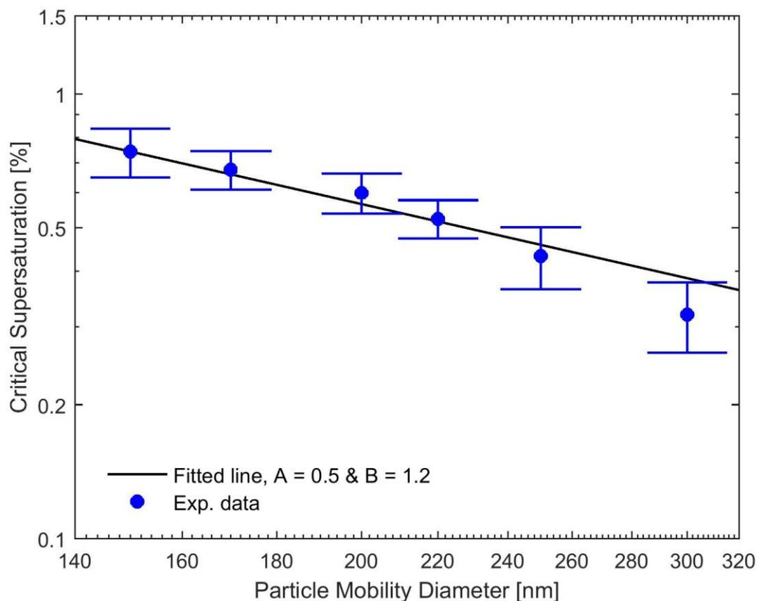
Fig. 4: Experimental and theoretical critical supersaturations for pure BC particles for different particle mobility diameters. The theoretical curve were calculated with Eq. 10 with  $A$  and  $B$  as fitting parameters. The experimental data was the average of two sets of experiments. Error bars represent the minimum vs. maximum values of supersaturations from the two data sets.
