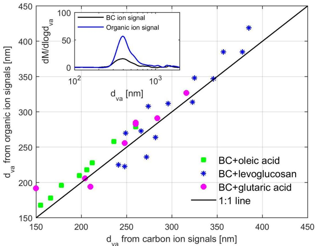
Fig. 3: Vacuum aerodynamic diameters ( $d_{va}$ ) from organic and carbon ions signals from SP-AMS for particles containing BC coated with various organic compounds. The inset represents mass size distribution vs.  $d_{va}$  extracted from BC and organic ion signals for monodispersed 200 nm BC particles coated by 27 nm levoglucosan. The coating thickness was estimated from the mobility size measurements by SMPS.
