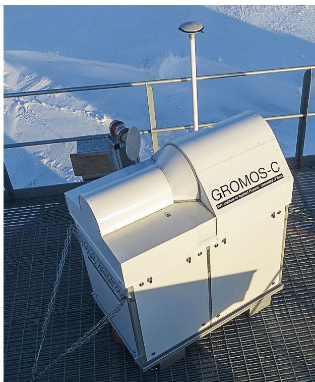
Figure 1. The ground based microwave radiometer GROMOS-C at the AWIPEV research base at Ny-Ålesund, Svalbard (79° N, 12° E). Observations in East and West direction are performed through a conical Teflon window with a rotating mirror inside the housing. North and Southward observations are performed via an external rotating mirror.
