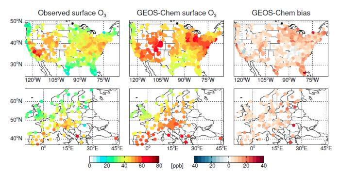
Figure 2. For both (top row) AQS network sites over the US and (bottom row) EMEP network sites over Europe: comparison of mean daytime (8:00–20:00 local time) (left column) observed and (middle column) GEOS-Chem simulated surface ozone concentrations for summer (JJA) 2010. Bias (simulated-observed) shown in right column.
