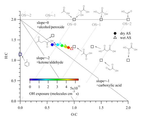
**Fig. 6.** Van Krevelen diagram of SOA derived from the photooxidation of toluene on initially wet and dry AS seed particles. SOA data are colored according to the OH exposure. Products identified in toluene-derived SOA are shown in boxes (Bloss et al., 2005; Hamilton et al., 2005; Sato et al., 2007). Average carbon oxidation states from Kroll et al. (2011) and functionalization slopes from Heald et al. (2010) are shown for reference.
