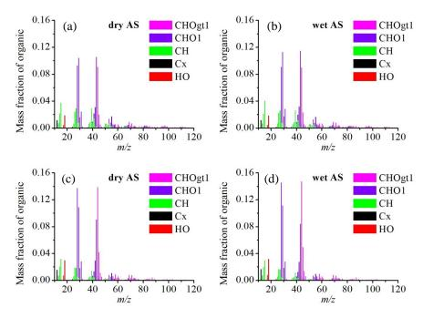
Fig. 4. High-resolution mass spectra of toluene-derived SOA on initially wet and dry AS at an OH exposure of (a, b)  $4.66\times10^{10}$  molecules cm<sup>-3</sup> s and (c, d)  $5.28\times10^{11}$ molecules cm<sup>-3</sup> s.
