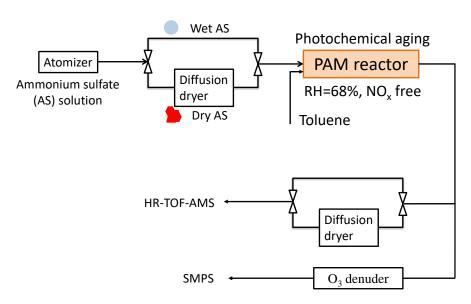
**Fig. 1.** Schematic of the experimental setup. The aqueous ammonium sulfate (AS) seed particles either passed through a diffusion dryer so that the phase of the seed particles could be altered or bypassed the diffusion dryer. Either wet or dry AS served as seed particles for the experiments.
