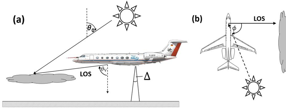
**Figure 1.** Illustration of the measurement geometry. (a) shows the side view with solar zenith angle  $\theta_0$  and the viewing angle  $\theta_v$ . The opening angle of the nadir looking radiance sensor of SMART is indicated by  $\Delta$ . Top view (b) shows the definition of the relative solar azimuth angle  $\phi$  between the line-of-sight (LOS) and the Sun.
