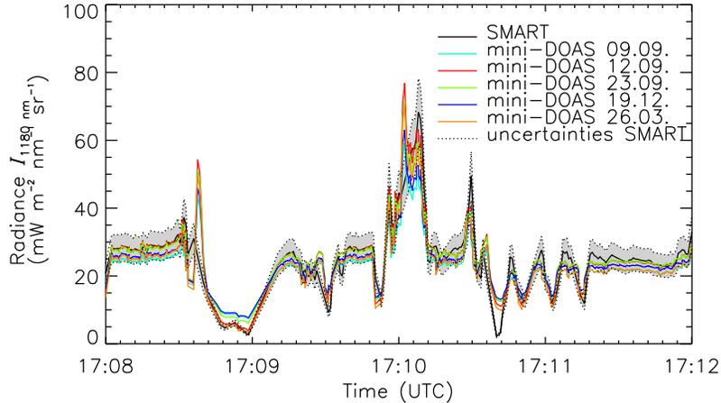
**Figure 10.** Time series of the nadir radiance of SMART  $I_{S,1180}^N$  and of the mini-DOAS  $I_{mD,1180}^N$  nadir channel at  $\lambda = 1180$  nm using different calibrations as indicated in the legend. The uncertainty range of SMART radiance is shaded gray.
