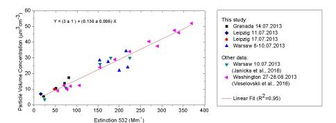
**Figure 10:** Scatter plot of the particle volume concentration as a function of the extinction coefficient at 532 nm. The red line represents the linear regression.
