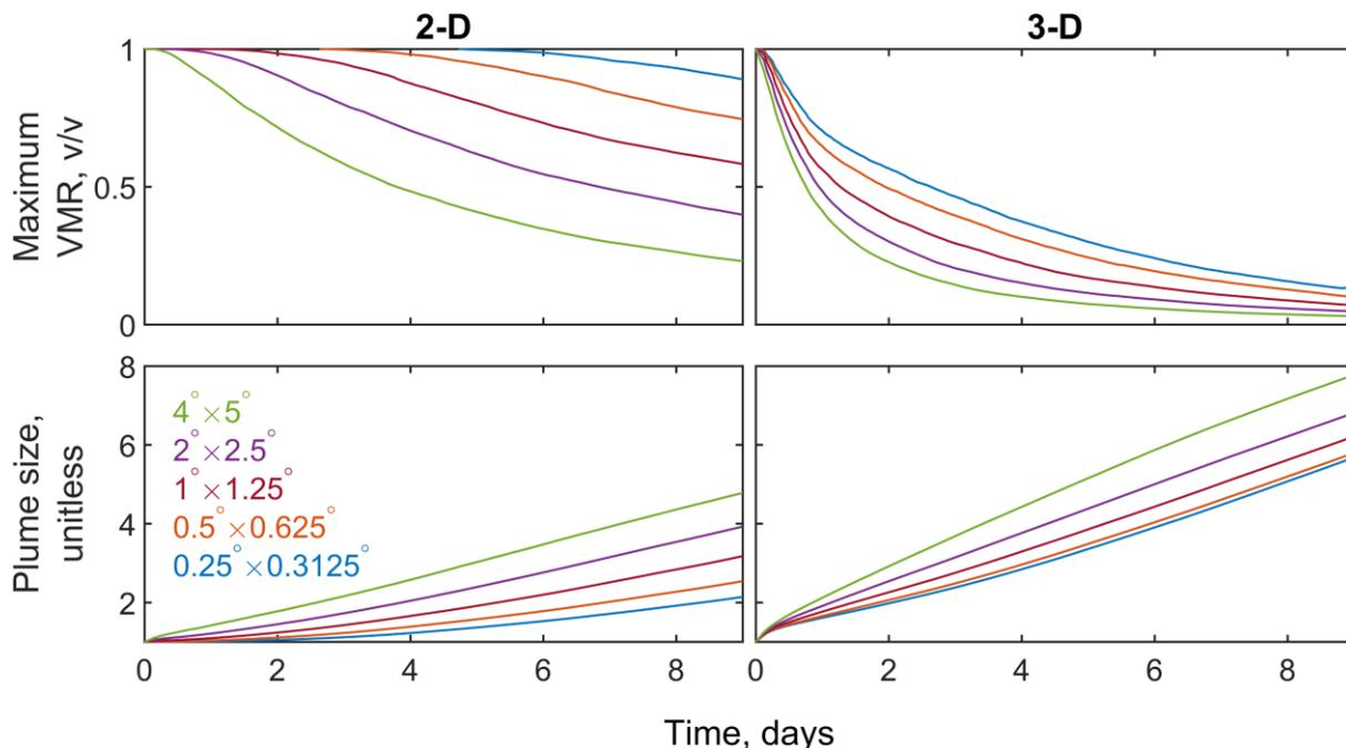
**Figure 6. Maximum VMR (top panel) and plume size (bottom panel) as a function of plume aging time. Values are global averages for the ensemble of 90 plumes in Fig. 1, and are shown for 2-D and 3-D simulations at the different horizontal grid resolutions indicated in the legend.**
