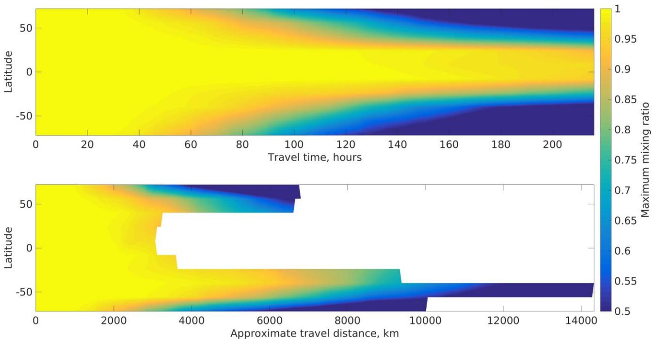
Figure C1: Maximum mixing ratio in a 2-D simulation. The upper plot shows the average for each latitude band as a function of travel time. The lower plot shows the average for each latitude band as a function of the approximate distance traveled by the plume. Due to the lower wind speeds in tropical regions, the final distance traveled within 9 days is smaller (~3,500 km).
