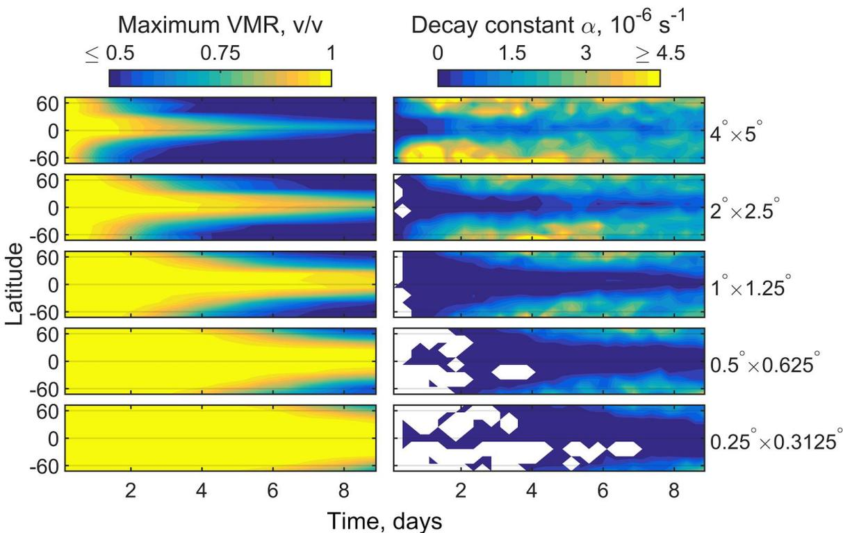
**Figure 3. Evolution with time of the maximum VMR and the decay constant  $\alpha$  for GEOS-Chem plumes initialized at different latitudes in a 2-D (horizontal) flow. White areas in the right panels correspond to no significant plume decay ( $\alpha \approx 0$ ).**
