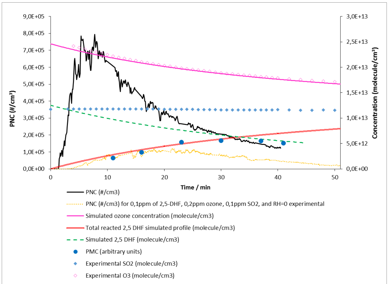
Figure 2. Temporal profiles for particles and gases. Initial concentrations: 0.5ppm of 2,5-DHF, 1ppm of O 3 , 0.5ppm of SO 2 and RH= 0.
