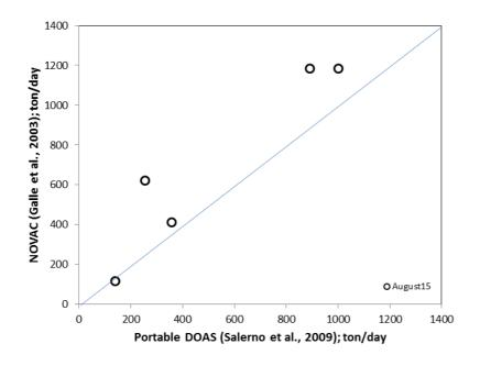
**Fig. 1.** Comparison of traverse mini-DOAS ('Portable DOAS') measurements with stationary scanning-DOAS ('NOVAC') measurements obtained on August 15 2015, evaluated with the methods mentioned in the manuscript.
