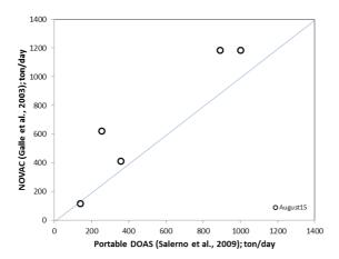
Figure RC1. Comparison of traverse mini-DOAS ('Portable DOAS') measurements with stationary scanning-DOAS ('NOVAC') measurements obtained on August 15 2015, evaluated with the methods mentioned in the manuscript. The correspondence is quite good and within the uncertainty of the measurements.
