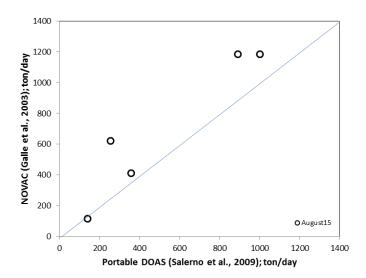
**Fig. 1.** Comparison of traverse mini-DOAS ('Portable DOAS') measurements with stationary scanning-DOAS ('NOVAC') measurements obtained on August 15 2015, evaluated with the methods mentioned in the manuscript.
