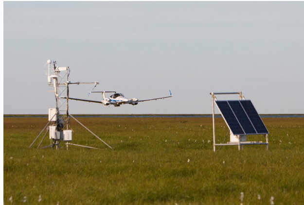
Figure 1. Picture of the FOCAL system flying near the NOAA/ATDD flux tower in North Slope, AK.
