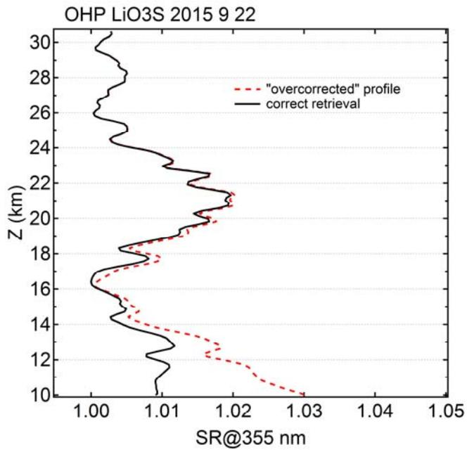
Figure AC1.1 Vertical profiles of scattering ratio @ 355 nm from OHP LiO3S lidar showing the effect of overcorrection for signal saturation on the aerosol retrieval in the lower stratosphere.
