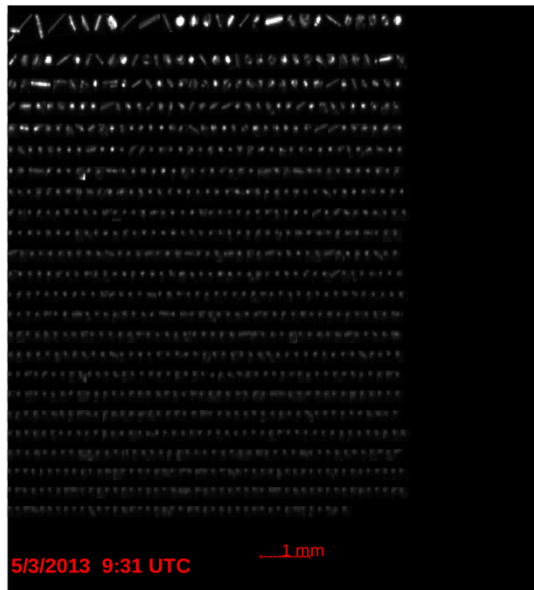
Figure R1. (From top to bottom and from left to right) Pictures taken from the ICE-CAMERA installed on the roof of the shelter where the HAMSTRAD and the aerosol Lidar are installed showing grains of ice crystals deposited over one hour on the surface of the camera in 2013 on: a) 4 March at 12:31 UTC; b) 4 March at 18:31 UTC; c) 5 March at 00:31 UTC; d) 5 March at 06:31 UTC and e) 5 March at 09:31 UTC. The 1-mm scale is indicated on each frame.
