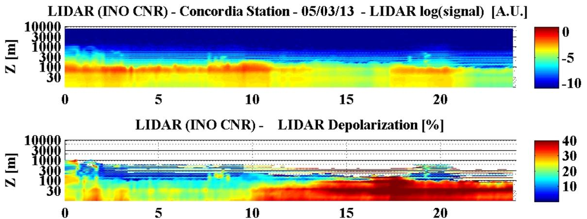
*Figure R8:* Time evolution of the Lidar raw signal (top) and depolarization (bottom) measured on 5 March 2013 above the Dome C station.
