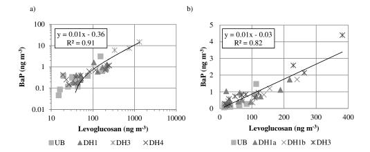
Figure 4: The linear correlation between BaP and levoglucosan concentrations in the urban background (UB) and suburban detached house areas (DH) in Helsinki metropolitan area for a) 24 h means in February 2012 and for b) monthly means in 2011. Panels (a) and (b) have been presented on logarithmic and linear scales, respectively. The number of data points was 41 (panel a) and 48 (panel b).
