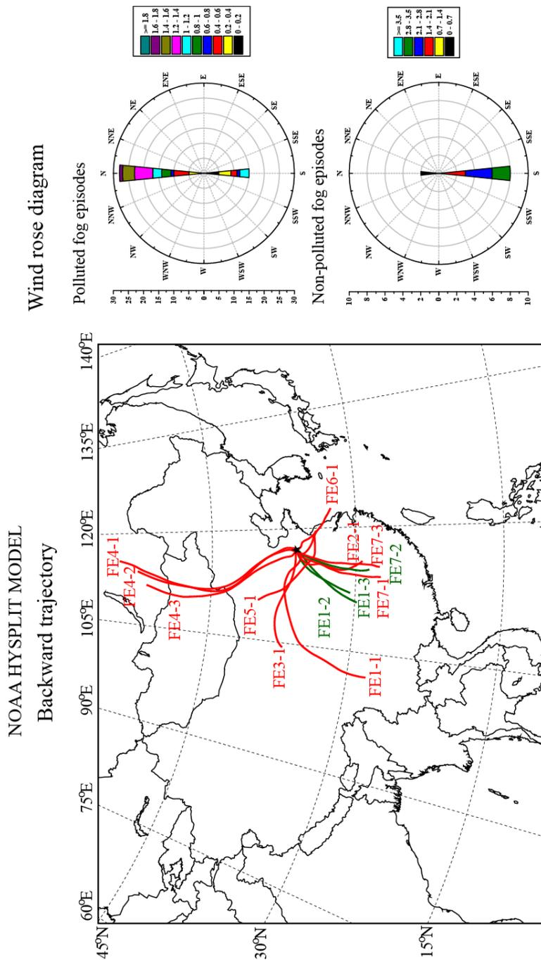
**Figure 7** Air mass transport pathways for the fog episodes using the Hybrid Single Particle Lagrangian Integrated Trajectory (HYSPLIT) model. 24-hour backward trajectories were calculated for air parcels arriving at 1534 m above sea level. Wind Rose Diagram of Study Area during sampling time.
