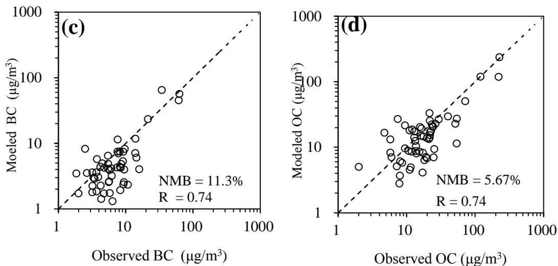
Fig. 2. Time series of the observed (dots) and simulated (line) (a) black carbon (BC) and (b) organic carbon (OC) mass concentrations ( $\mu\text{g m}^{-3}$ ) at the Suixi site. Scatterplots of simulated (c) BC and (d) OC mass concentrations ( $\mu\text{g m}^{-3}$ ) and corresponding observed values. NMB and R represent normalized mean bias and correlation coefficient, respectively.
