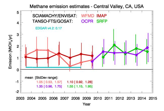
**Figure 10.** Methane emission estimates for Central Valley area in California, USA, as defined for this study (see Fig. 9 and Tab. 2). The blue line shows the EDGAR v4.2 (annual) anthropogenic methane emissions as computed for the Central Valley source region.
