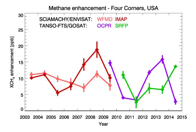
Figure 7. Methane enhancements over the Four Corners area for all years and all four satellite data products used in this study. The error bars show the standard deviation of the methane enhancements obtained by varying the size and shape of the surrounding area.
