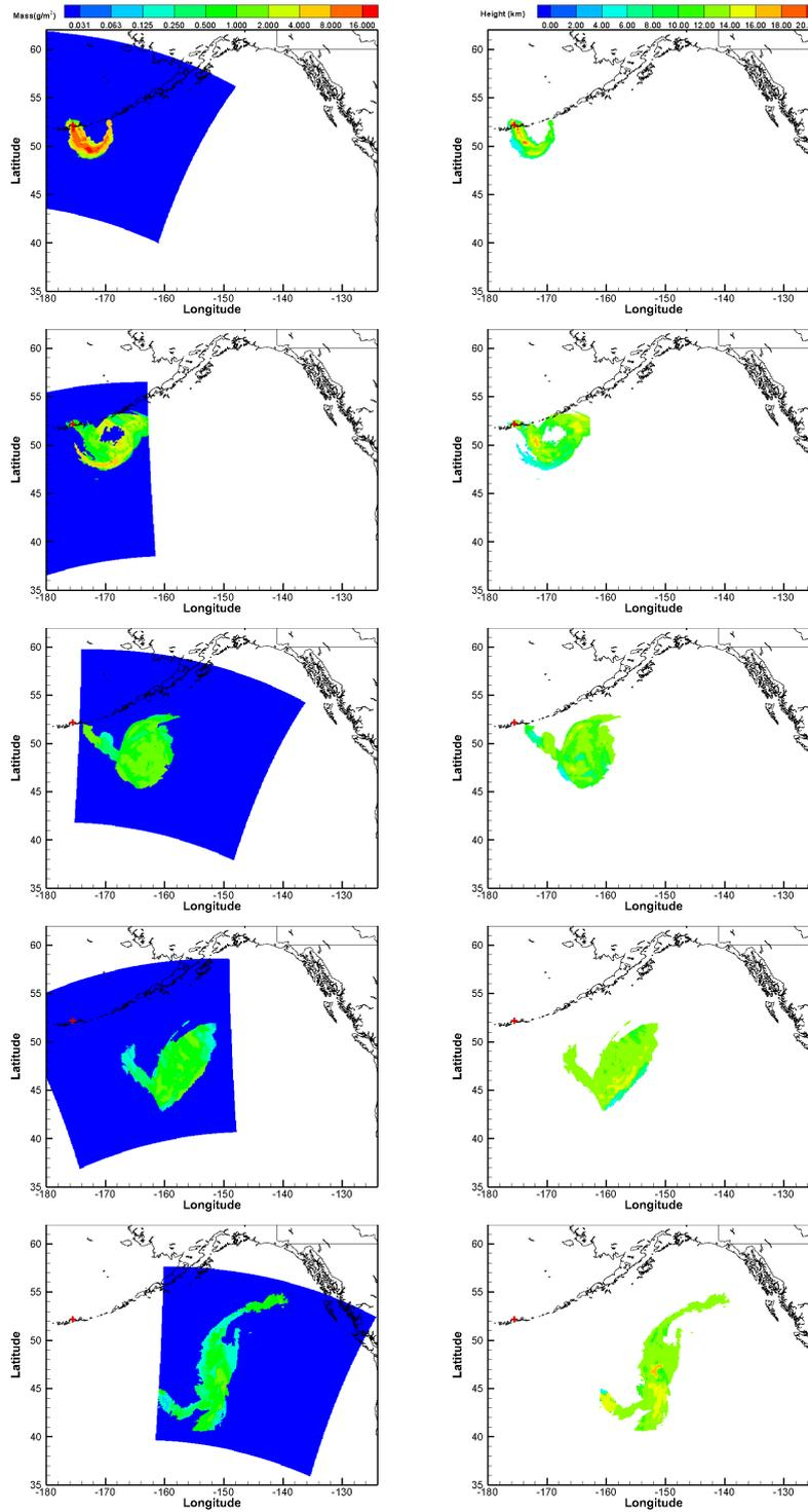
**Figure 1.** MODIS volcanic ash mass loadings (left) and ash cloud top height(right) listed from top to bottom following their observation time (see Table 1 for detail). “+” shows the location of Kasatochi volcano ( $52.1714^{\circ}\text{N}$ ,  $175.5183^{\circ}\text{W}$ ). Note that the satellite observations to the left of the map domain are not used in this paper.
