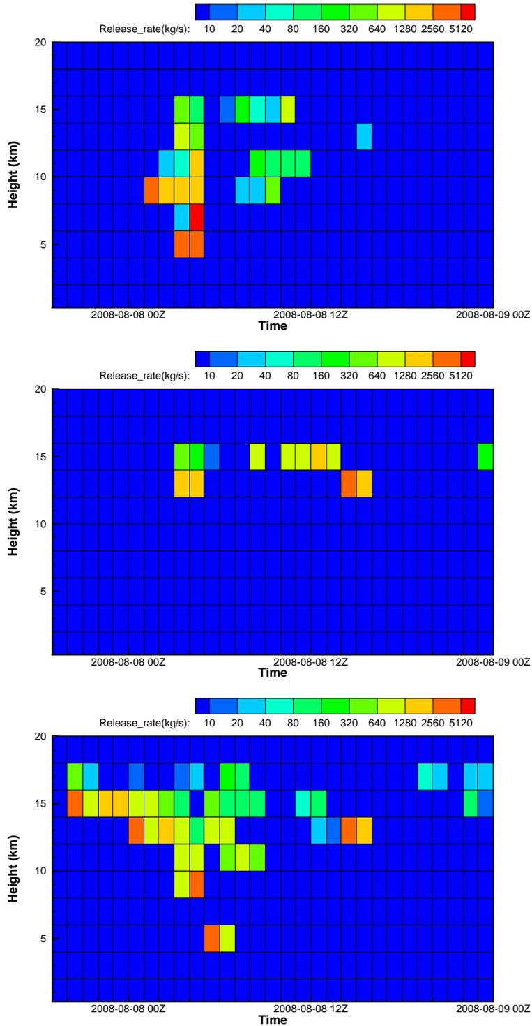
**Figure 4.** Volcanic ash release estimates with different options in model mass loading calculation. From top to bottom: integrating from surface to cloud top (same as Figure 3 top), calculated for a single layer where the cloud top height resides, and integrating over three layers centered at the cloud top layer.
