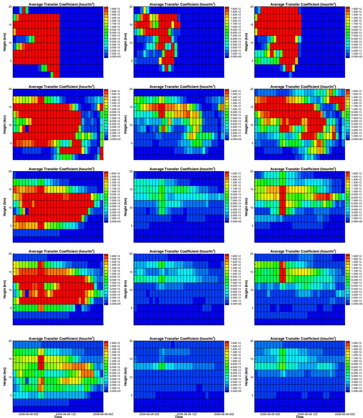
**Figure 2.** Averaged TCMs using GDAS meteorological data with three different options in calculating model mass loadings (Column 1: integrating from surface to observed cloud top; Column 2: calculated for a single layer where the observed cloud top height resides; Column 3: integrating over three layers centered at the observed cloud top layer). Rows 1-5 (from top to bottom) correspond to observations G1-5.
