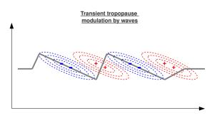
**Figure 2.** Schematic of transient tropopause modulation by an idealized wave with westward vertical tilt, as a snapshot of the wave's temperature anomalies (dashed contours: positive red, negative blue) and the undulating tropopause (thick and solid grey line).
