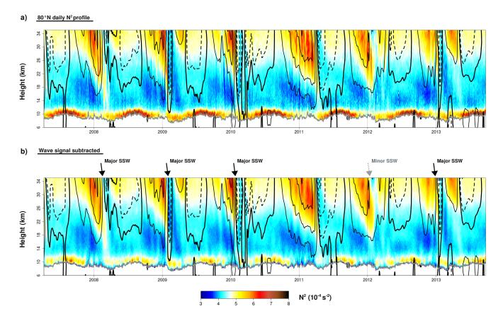
**Figure 7.** As in Fig. 5, but for 80°N. Major and minor SSWs are marked above Fig. 7b. First easterly wind contour (dashed line) at -3m/s for better visibility. The rest of wind contours are 10m/s intervals as in Fig. 5.
