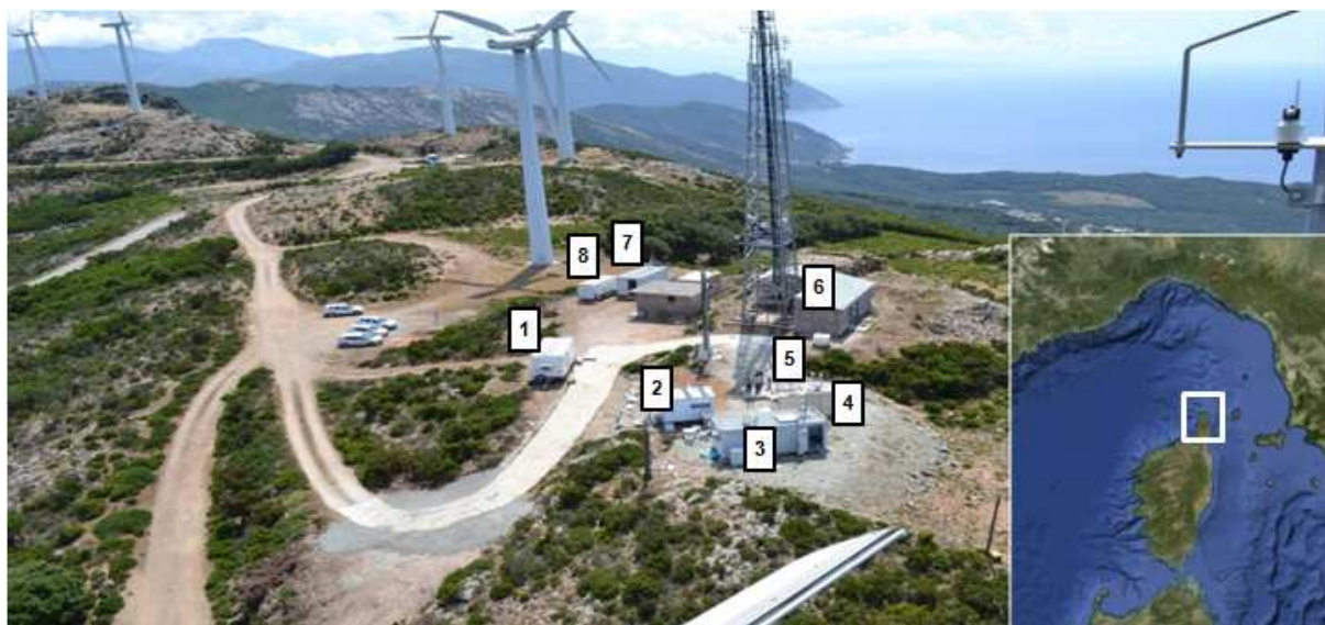
Figure 1. Field site top-view, Corsica, France (42.97°N, 9.38°E, altitude 533 m). Measures: 1. PTR-MS, online and offline chromatography for trace gases analysis; 2. OH reactivity; 3. NO x , O 3 , aerosols composition and black carbon; 4. Meteo, and particles microphysics; 5. HCHO, trace gases and radicals; 6. CO, CO 2 , CH 4 ; 7. Trace gases and particle filters; 8. Particles physics. The photo was taken during the installation of the instruments.
