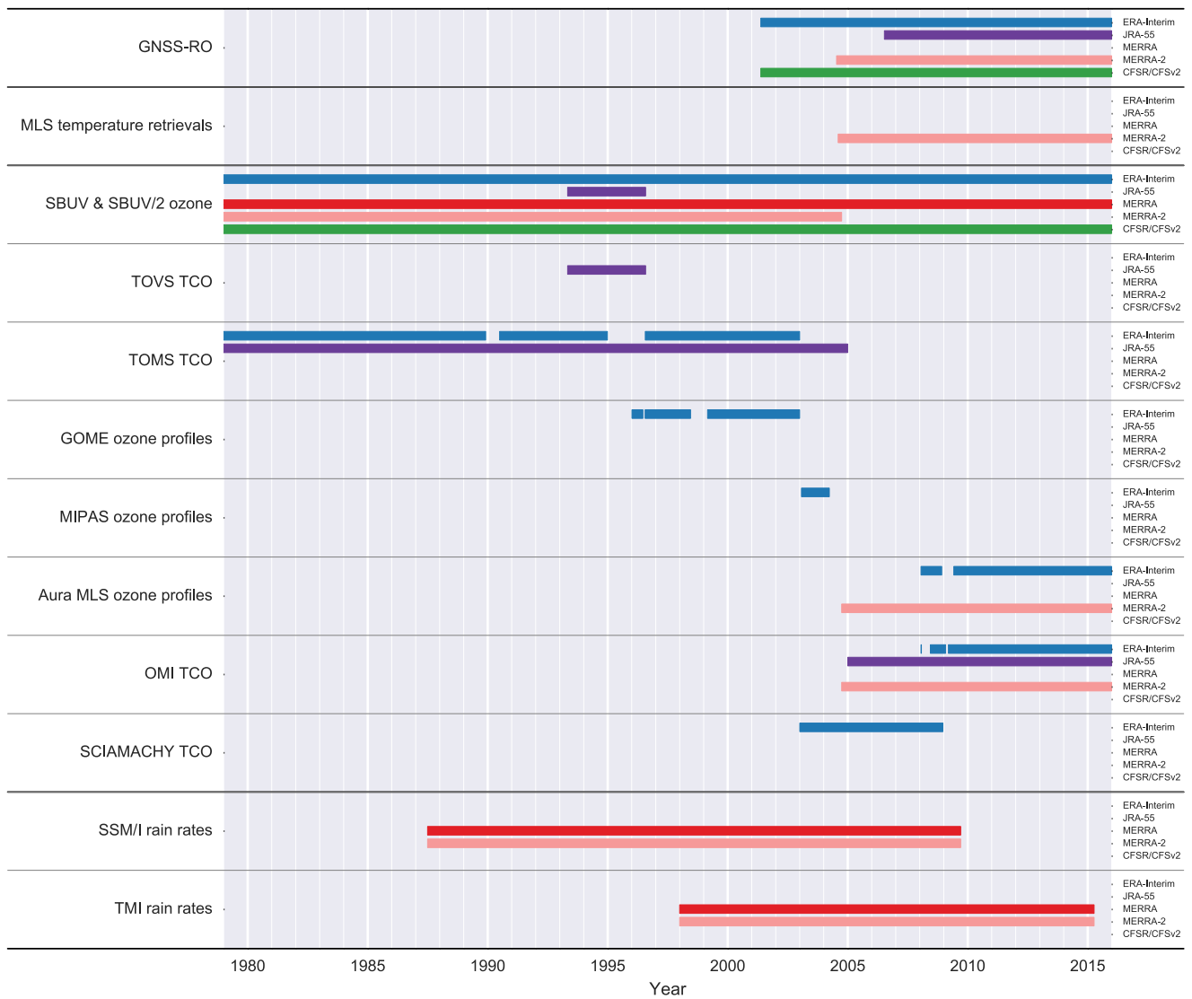
Figure 109. As in Fig. 65, but for other types of satellite observations assimilated by the reanalysis systems, including GNSS-RO (or GPS-RO), satellite temperature and ozone retrievals, and rain rates derived from microwave imagers. Aura 5 MLS temperature retrievals are assimilated by MERRA-2 only in the upper stratosphere at pressures less than 5 hPa. SBUV and SBUV/2 are used by reanalyses to supply ozone profile information, TCO, or both. JRA-55 assimilates only TCO, ERA-Interim assimilates only profiles, and CFSR, MERRA, and MERRA-2 assimilate both TCO and profiles. See Appendix A for acronym definitions.
