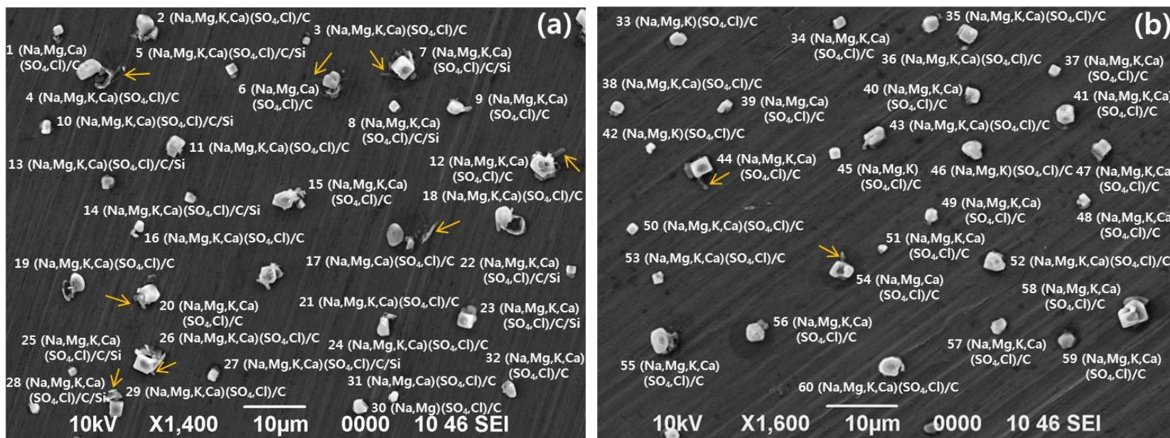
Figure 2. Secondary electron, molecular Raman map, and elemental X-ray map (overlaid on SEIs) images of two typical (a) summertime and (b) wintertime SSAs.
