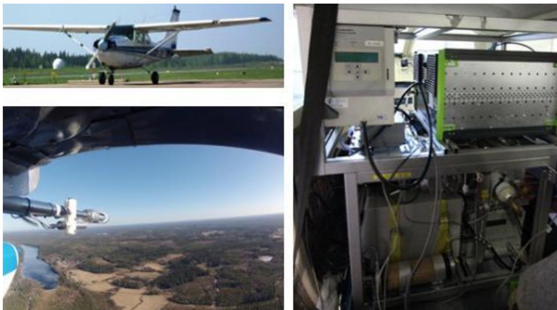
**Figure 1.** Upper left panel: The instrumented Cessna 172 aircraft. Down left panel: The sample air inlet under the wing, and an aerial view towards Hyytiälä measurement station. Right panel: Measurement instruments on-board.
