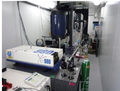
Figure 1. Mie lidar and ozone DIAL (right) were installed in the container at the left on the ground (left).
