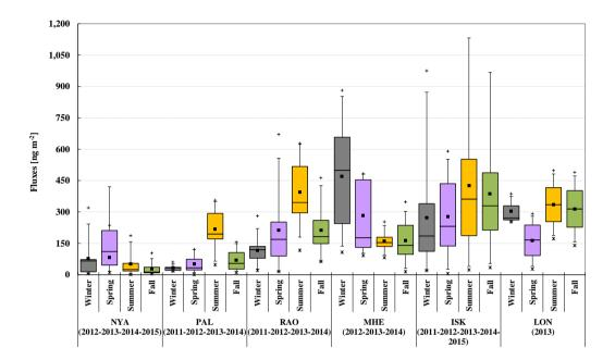
Figure 4. Seasonal distribution of time sampling flux-weighted (by 15 days reference) at the European GMOS sites from 2011 to 2015. Each box includes the median(midline), mean (, 25th and 75th percentiles (box edges), 5th and 95th percentiles (whiskers), minimum (\*) and maximum (+).
