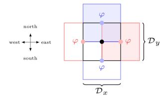
Figure 11. Averaging concept for the determination of larger-scale forcing terms from COSMO model output. The shifted domains (red/blue) are used for the calculation of larger-scale gradients of  $\phi \in \{\theta_{\text{l,LS}}, q_{\text{t,LS}}\}$ . The centered averaging domain (black) is used for the calculation of all other larger-scale quantities.
