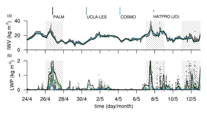
**Figure 8.** Temporal evolution of integrated water vapor IWV in panel a and liquid water path LWP in panel b. An overview of the measurements and abbreviations is given in Tab. 1. Gray and green shading in panel b denote twice the standard deviation of LWP in PALM and UCLA-LES, respectively. Stippled highlighting as in Fig. 6.
