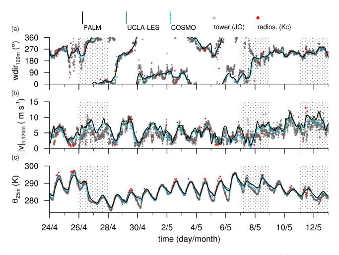
Figure 7. Temporal evolution of wind direction at 120 m height wdir<sub>120m</sub> in panel a, wind speed at 120 m height  $|v|_{h,120m}$  in panel b and potential temperature at 25 m height  $\theta_{25m}$  in panel c. An overview of the measurements and abbreviations is given in Tab. 1. Stippled highlighting as in Fig. 6.
