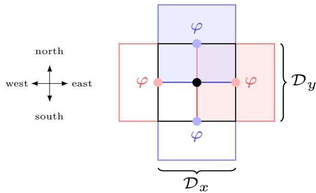
**Figure 11.** Averaging concept for the determination of larger-scale forcing terms from COSMO model output. The shifted domains (red/blue) are used for the calculation of larger-scale gradients of  $\phi \in \{\theta_{i,LS}, q_{i,LS}\}$ . The centered averaging domain (black) is used for the calculation of all other larger-scale quantities.
