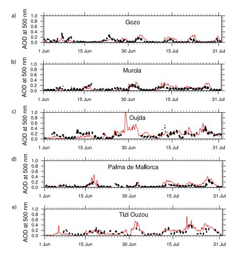
**Figure 2.** Temporal evolution of dust AOD at five different stations (see Fig. 1) located along frequent dust transport routes. Dust AODs calculated from 3-hourly COSMO-MUSCAT output for June and July 2013 is represented by the red line, AERONET level 2.0 coarse mode AOD retrievals from sun-photometer measurements are shown in black. COSMO-MUSCAT dust AODs are calculated for the grid cell corresponding to the AERONET measurement site.
